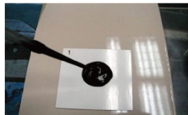
(1) 使用10% carbon solution (10g碳黑顏料+90g水)滴在試驗板上 Apply 10% carbon solution (10g of carbon blackpigment +90g of water) and drop it on the test specimen.
