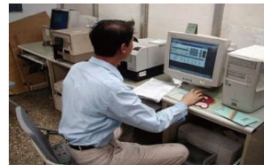
以電腦測量原色板與汙染色板之色差數值 Measure the color difference between the original and polluted color palettes with computer.
