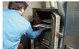
(2) 置於80°C恆溫箱烘烤1小時 Place it in the thermostated container at 80°C and bake for 1 hour.
